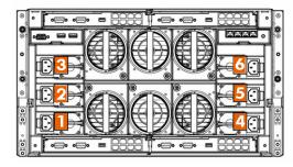
The new, high efficiency HP c3000 power supplies provide greater than 90 percent efficiency in AC to DC conversion. These power supplies use the ProLiant universal form factor so they can also be used in other ProLiant servers. Each AC power supply ships with a standard power distribution unit (PDU) power cord (C13 to C14). By purchasing proper wall outlet cords, users can connect the power supplies to standard wall outlets.
